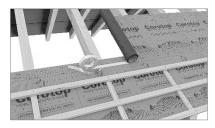
5. In order to eliminate draughts in the roof baffle, it is recommended (in case of roofs with pitches below 20° it is required) to bond the membrane overlaps with the Corotop Mix tape.
